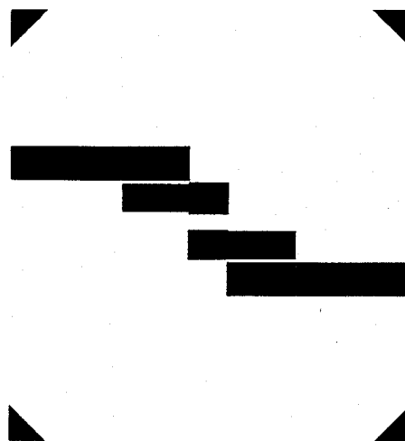
Fig. 8. Layout of a microstrip coupled line bandpass filter. Substrate: RT/Duroid, \epsilon_r = 2.33 , h = 0.79 mm; scale: 2:1.
